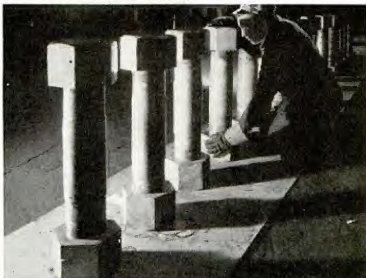
These 315-pound bolts will join two sections of a steel shaft for a giant generator. The night workman just finished painting bolts
